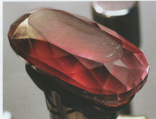
Fig. 6.29 Completed faceting of crown on oval.
