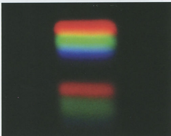
Fig. 6.34 Doubled images seen when the table facet of a zultanite is held close to the eye while viewing a light source. “ Visual Optics ” identification method and photo by Alan Hodgkinson.
