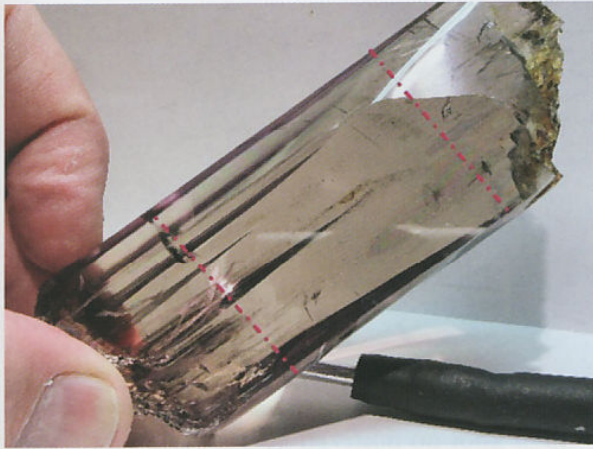
Fig. 6.14 Saw cut outlined to remove bad parts.
