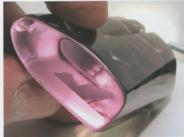
Fig. 6.17 Cleavage parting in interior at small end.
