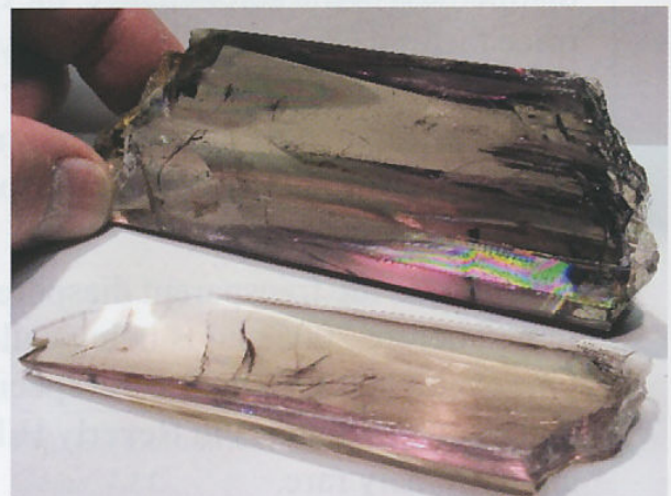
Fig. 6.13 Cleavage separated from main section.
