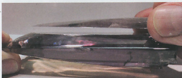
Fig. 6.12 Side view of separated cleavage on large crystal.
