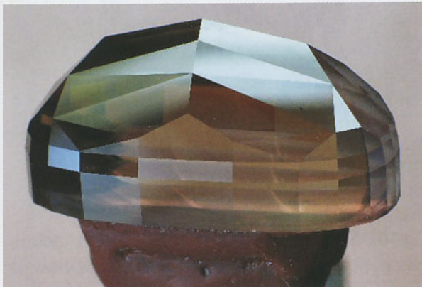
Fig. 6.28 Polished fully faceted pavilion on long oval.
