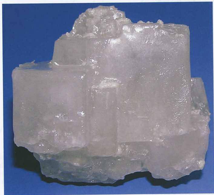
Figure 7. Calcite crystals of pseudocubic rhombohedral habit are a common accessory mineral in the diaspore-rich hydrothermal veins. This specimen is 8.5 cm wide. Murat Hatipoglu photo.
